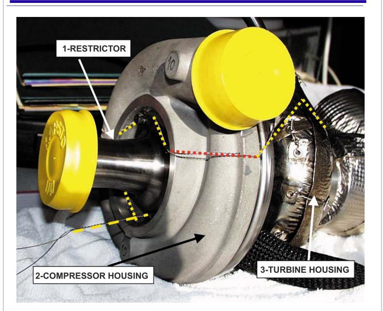
The articles 254-6.1 (Group N) and 255-5.1.8.3 (Group A) from Appendix J state: The restricot must be made from a single material and may be pierced solely for the purpose of mounting and sealing, which must be carried out between the mounting screws, between the restrictor (or the restrictor/compressor housing attachment), the compressor housing (or the housing/flange attachment) and the turbine housing (or the housing/flange attachment) (see drawing 254-4).
